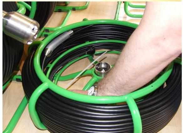
Pull the Molex connector slightly from the coiler and hold in place with a small screwdriver
