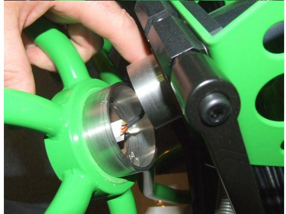
Fit the T710 coiler inside the T804 coiler. Ensure the T710 clamps are facing downwards
