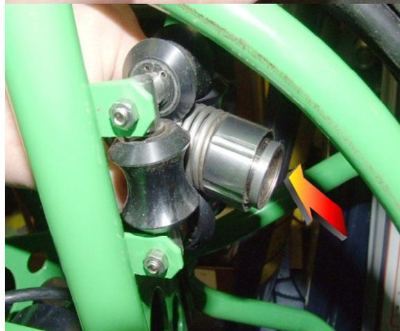
Apply the coiler brake so that the coiler cannot rotate
