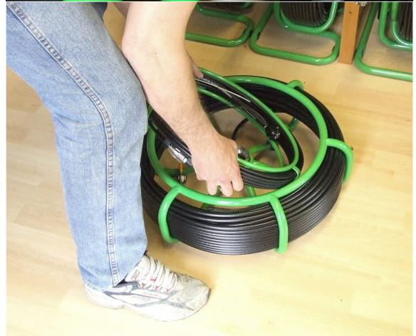
Push the T710 clamps onto the T804 coiler
