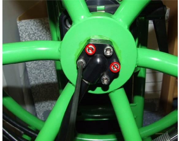
Release the brake and carefully and slowly pull the coiler away from the hub. Once access is possible disconnect the Molex connector.
