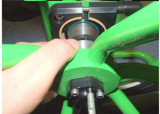
Carefully push the coiler onto the hub assembly. Release the brake further if the parts do not mate smoothly.
