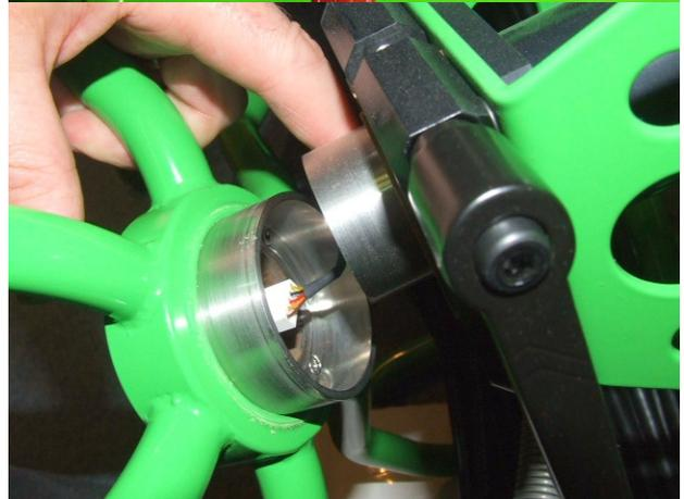
Use an Allen driver to align one of the Allen bolt bores with the corresponding threaded hole in the hub assembly
