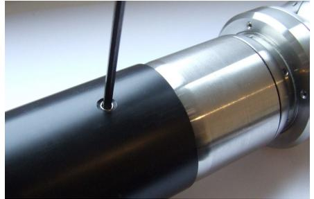
Unscrew camera from T804 termination and internal adaptor tube.
