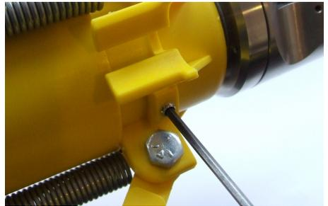
Set the skid to the correct diameter for the pipe being surveyed and then lightly tighten the friction bolts to hold the skid in position. For pipes between 150mm-200mm, use the small wheel set.
