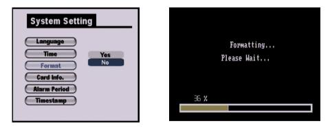
When formatting is complete the screen will momentarily show 'Format OK' and the system will automatically return to normal operation after 2 minutes.
