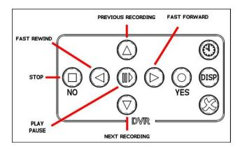
**The screen will momentarily show 'DVR PLAY MODE'** and the last video or snapshot will be shown. Use the 'Fast Forward' and 'Fast Rewind' buttons if required (these have no function when a snapshot is shown).
