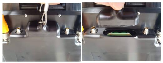
Insert the SD card with LABEL UPWARDS.
