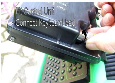
7) Connect Keyboard connector to the Control Unit
