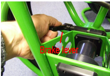
10) Adjust the brake lever so that the coiler can be turned with a little resistance
