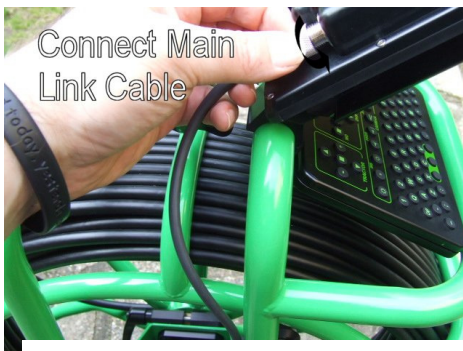
8) Connect Link Cable to Control Unit
