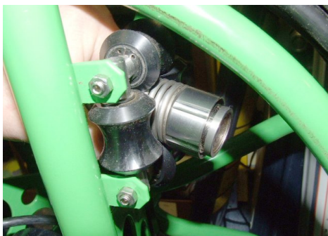
11) Cut tie-wrap and remove soft cover from termination. Thread the termination through the Rod Guide
