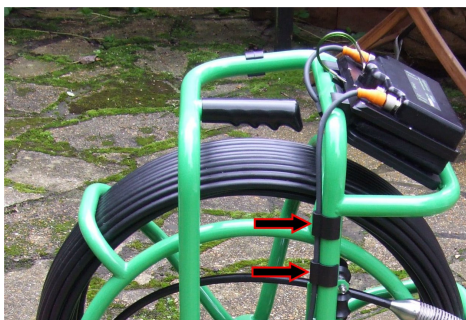
9) Fit two of the cable clips as shown to secure the Link Cable. There are 4 clips supplied with the system.
