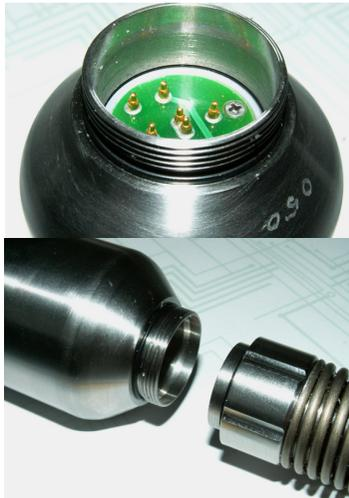
Prior to fitting, the rear of the camera and rod end connector should be checked for dirt and moisture and cleaned if necessary.
