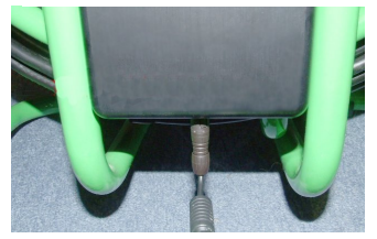
The Power Cell can be charged whilst fitted to the frame if preferred DO NOT OPERATE DURING CHARGE
