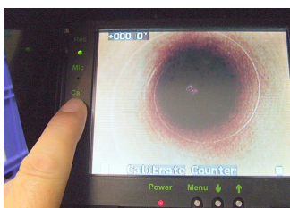
Press the Rod Counter button until the display shows 'Counter Calibrated'
