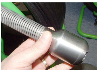
Fit camera to Rod Termination
