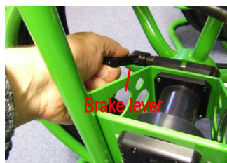
Adjust the brake to supply a small amount of friction. You are now ready for surveying
