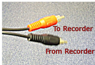
Connect to external recorder. The T804 will select video from the recorder automatically
