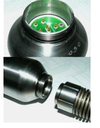
The camera is then screwed onto the rod end connector until fully hand tight. No tools are required to tighten the locking collar which is prevented from unscrewing by the small O ring at the end of the connector thread.
